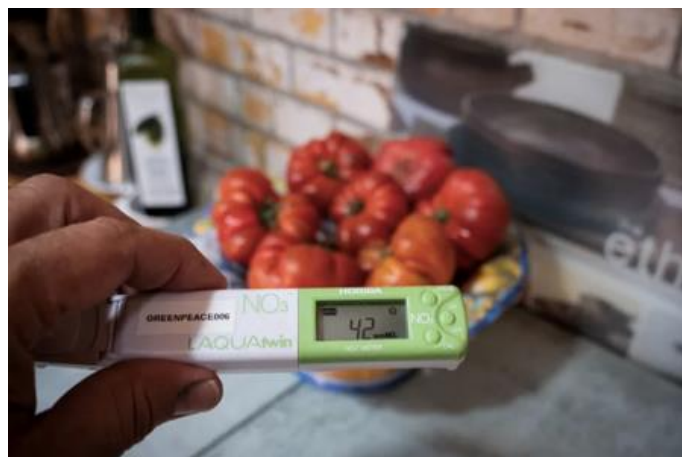
Picture 1. The LAQUAtwinNO3-11 device used to measure nitrate concentration in water samples. © Foto: Greenpeace
